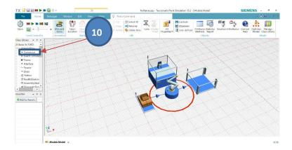
**11.** From *User Interface* toolbox menu, select *Display* places near **Source** and **Buffer**, double click on each display object then set *Comment* property to *Input*: and *Output*:
