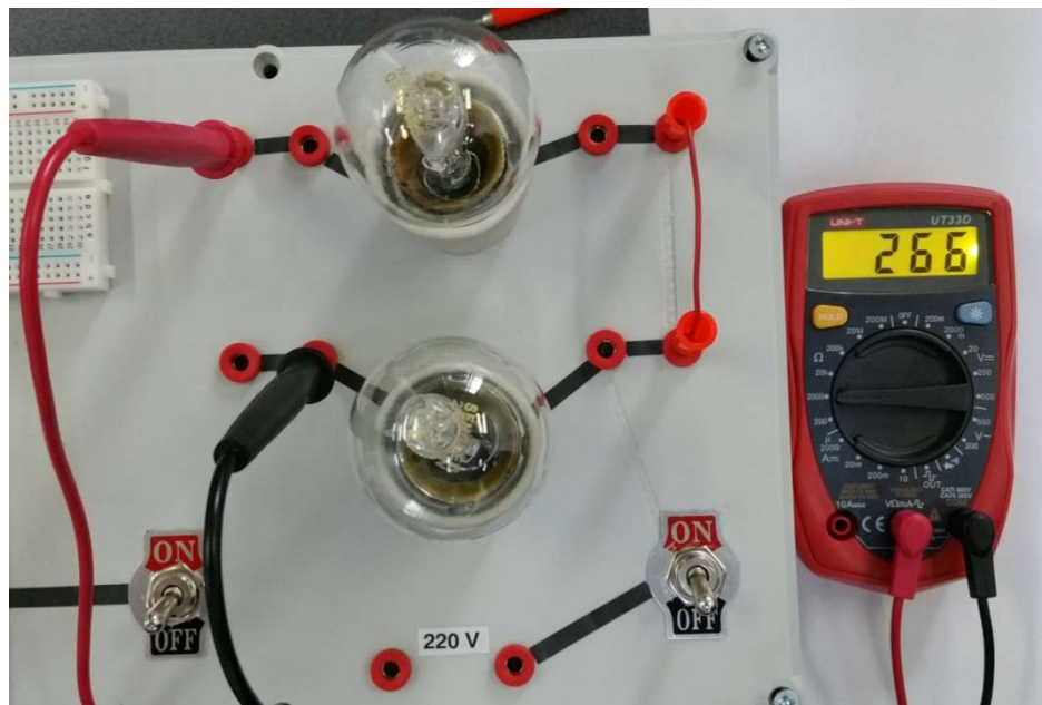
Fig. 1.12: Measuring the series circuit total resistance
