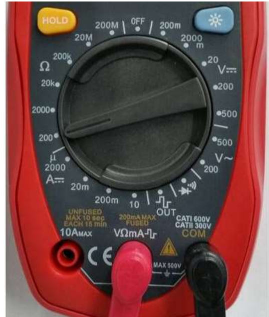
Fig. 1.9: Rotary switch position and test leads connections
