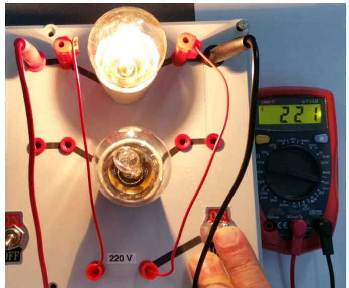
Fig. 1.16: Measuring the voltage across LB2 powered alone
