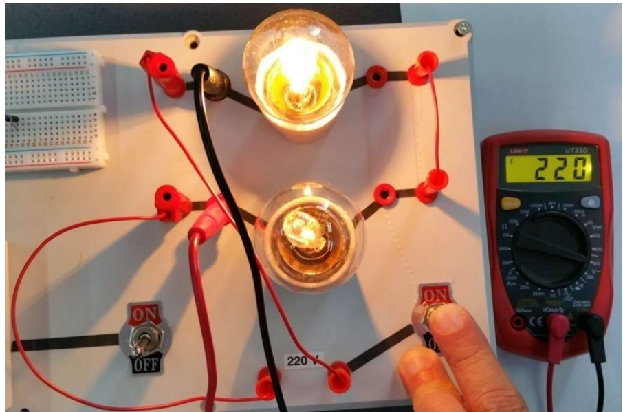
Fig. 1.17: Measuring the voltage across the whole series circuit
