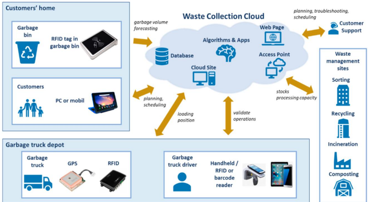
Figure xx. The Waste Collection Cloud and its connections with the cyber-physical waste collection system including customers, garbage trucks, waste management sites and customer support (Bányai et al., 2019)
