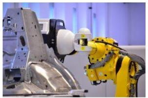
Robot mounted Laser Radar mounted measures studs on a car body component
