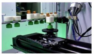
Automated CT inspection analyzes batches of connectors for geometrical deviations
