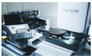
Semiconductor wafers automatically inspected on VCMM with a loading mechanism
