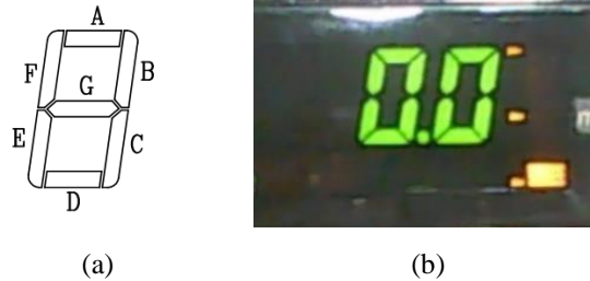
Fig. 1. (a) The seven-segment format, (b) LED seven-segment display.
