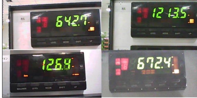
Fig. 2. Difficulties in the detection and recognition process (skew image, light disturbances image, blurry image, and intricate background image).
